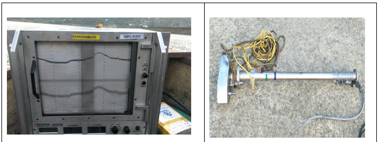
Fig.11: Echo sounder read out unit with sensor
