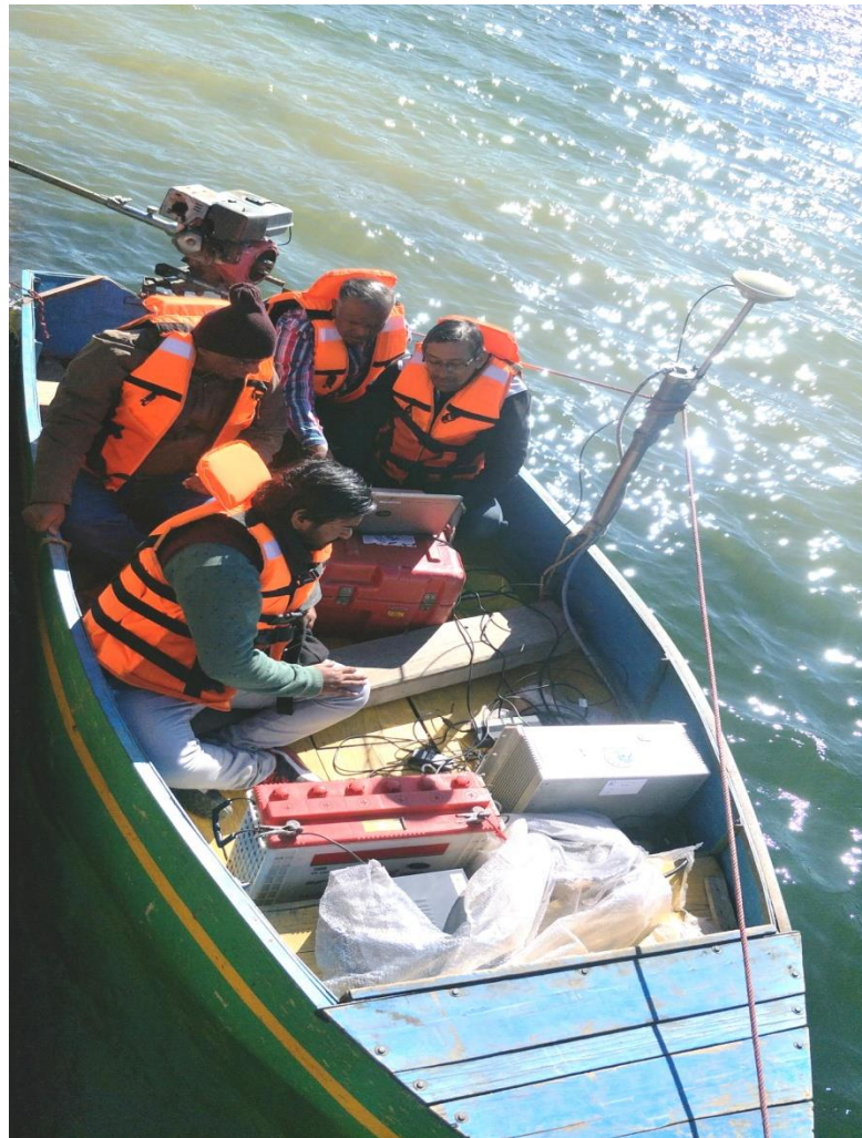
Fig.10: Survey Boat with GPS Antenna along with Mechanical Fixture for Eco-sounder
