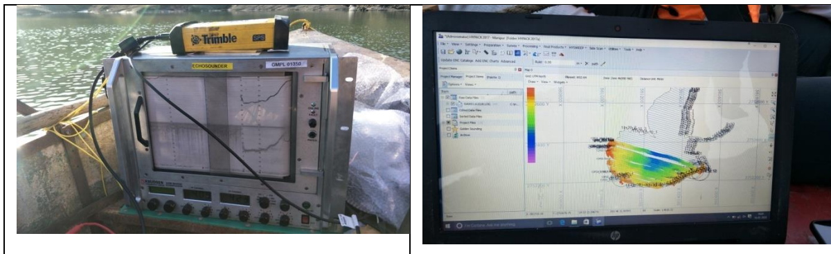
Fig.8 :Echo-sounder with Laptop for logging real-time data acquisition- IBS Equipment
